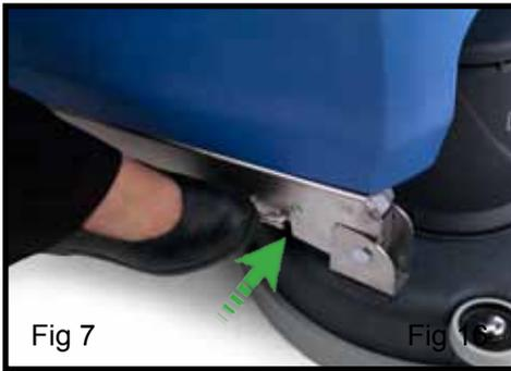
To tip the deck into the down position (Operating mode). Press in the brush deck locking bar (Fig 7) and rotate the brush deck (Fig 8).
