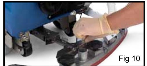
The lifting strap is held by a detent pin (Fig 10).
