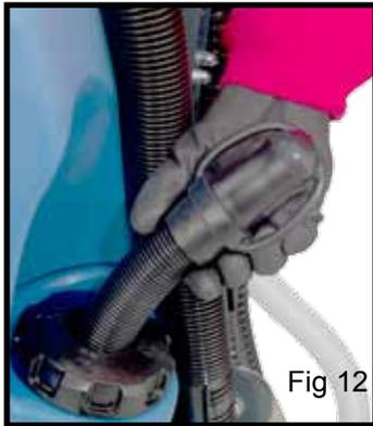
To fill the clean-water tank, use the FLEXI - FILL pipe from either a tap or hose pipe (Fig 12).
