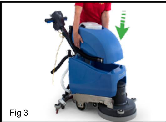
Fit the top tank to the machine (fig 3).
