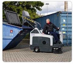
Hydraulic, high-dump hopper provides easy and safe disposal of large debris volume
