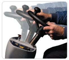
Adjustable seat and tilt steering wheel provide comfort for operators
