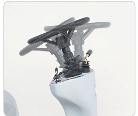
With an adjustable steering column, and heel and toe pedals for directional control, the rider sweeper provides ergonomic and safe operation.
