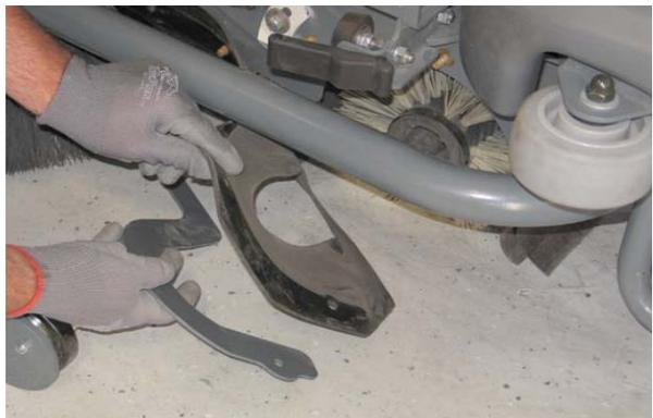
7. Remove the cylindrical brush and replace with a new brush.
