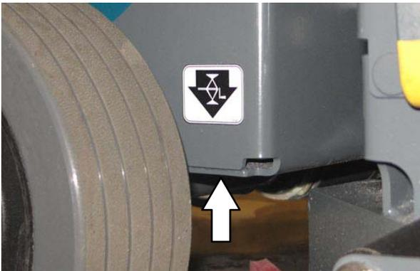
**FOR SAFETY: When servicing machine, block machine tires before jacking machine up. Use a hoist or jack that will support the weight of the machine. Jack machine up at designated locations only. Support machine with jack stands.**
