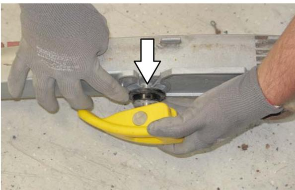
10. Install the rotated or new squeegee blade into the outer frame. Be sure the squeegee is completely slid down onto each tab on the outer frame.
