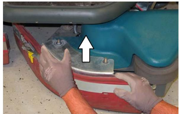
4. Loosen the retaining band latch.
