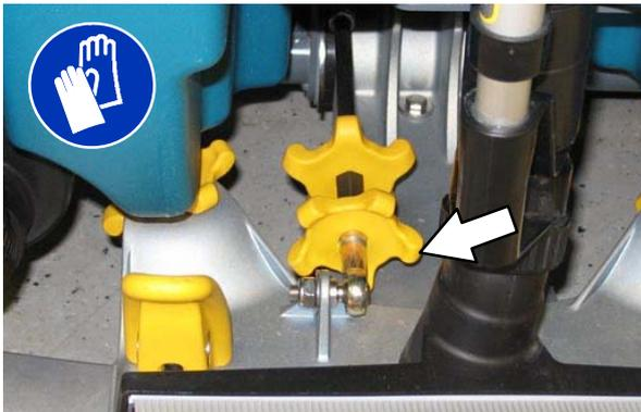
5. Turn the squeegee tilt adjust knob counter-clockwise to decrease the deflection at the ends of the squeegee blade.
