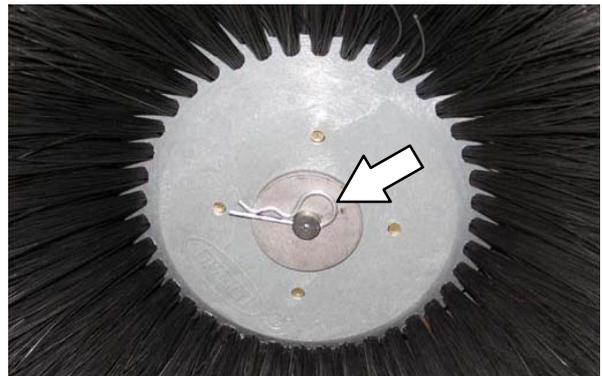
5. Remove the side brush from under the Pre-Sweep assembly.
