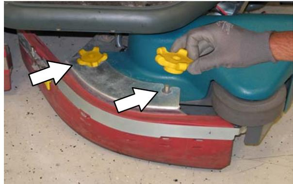
4. Squeeze the spring handles and let the side brush drop to the floor.
