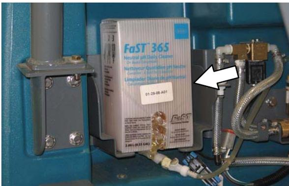
3. Remove the perforated knock outs from the new FaST-PAK carton. DO NOT remove the bag from the carton. Pull the hose connector from the bottom of the bag and remove the hose cap from the connector.
