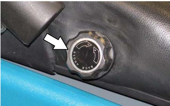
The weight adjustment knob controls the firmness of the operator seat. Use the gauge next to the weight adjustment knob to help determine seat firmness.
