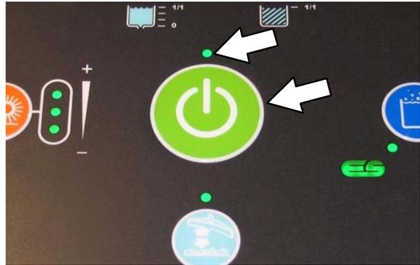
9. Repeatedly press the *Solution increase* button (+) until the solution flow is at the highest setting.
