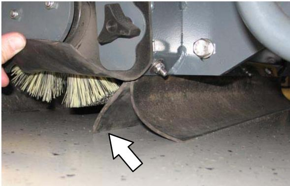
Check the skirt for damage and wear after every 50 hours of operation.
