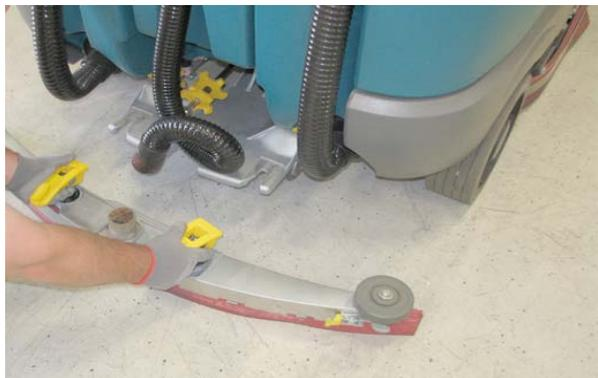
5. Loosen the retainer latch and remove the retainer from the squeegee assembly.
