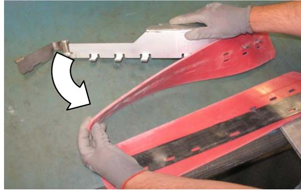
*NOTE: Observe which squeegee slots were installed on the squeegee frame before removing the squeegee.*
