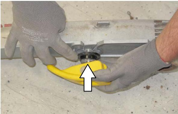
13. Place the rotated or new squeegee blade onto the inner frame. Be sure the squeegee is securely attached on each tab on the inner frame.
