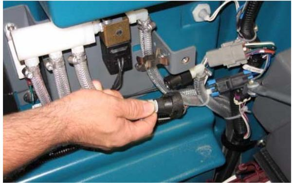
5. Connect the drain hose to the ec-H<sub>2</sub>O manifold hose disconnected from the outlet hose in the previous step.
