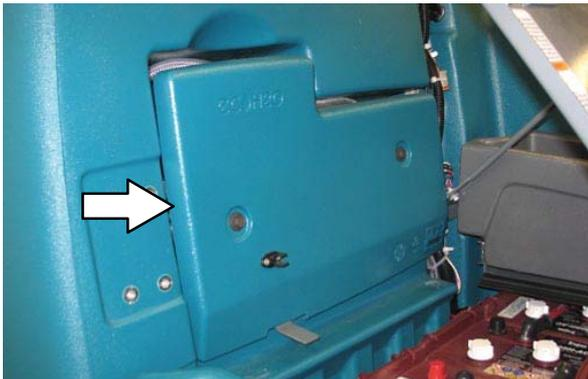
3. Remove the drain hose from the *ec-H2O* compartment.
