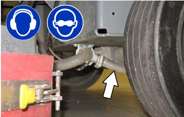
3. Use between 13.8 – 27.6 kPa (2 – 4 psi) of compressed air to blow remaining solution from the disconnected hose.
