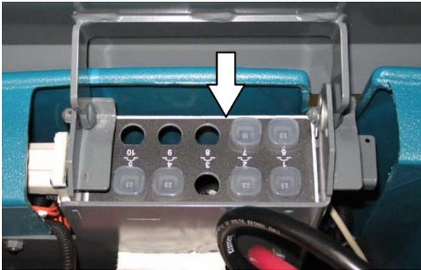
Circuit breakers 11 through 19 are located on the electrical panel.
