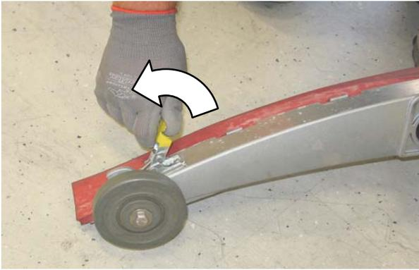
8. Remove the inner frame from the outer frame.
