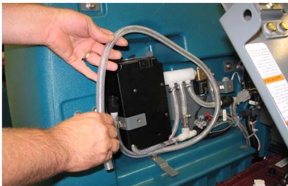
4. Disconnect the outlet hose to the scrub head from the *ec-H2O* manifold hose.
