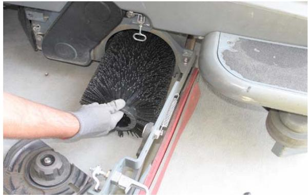
5. Position the brush with the *double row end towards the scrub head opening*. Guide the new brush onto the drive hub.
