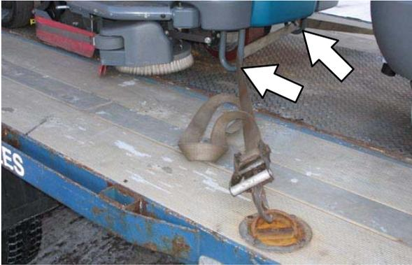
The rear tie-down locations are the holes in the frame.
