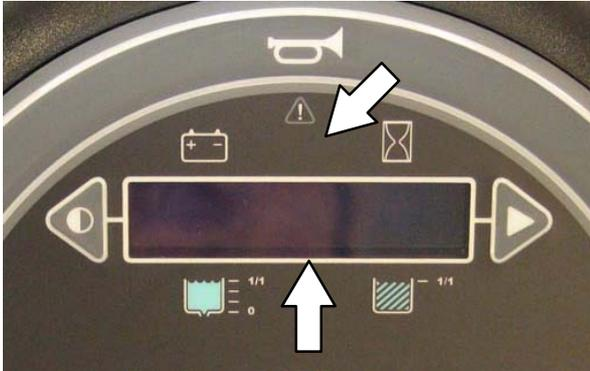
The LCD will display a fault code. If there is more than one fault, each fault code will alternately display.
