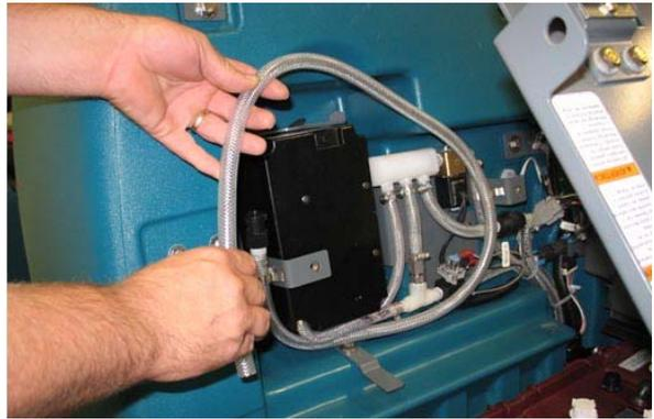
8. Disconnect the outlet hose to the scrub head from the ec-H<sub>2</sub>O manifold hose.
