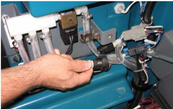
9. Connect the drain hose to the ec-H<sub>2</sub>O manifold hose disconnected from the outlet hose in the previous step.
