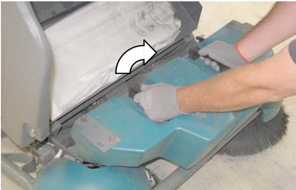
3. Reinstall the debris hopper into the Pre-Sweep assembly.
