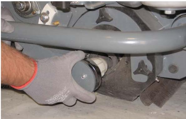
5. Remove the three knobs holding the Pre-Sweep side skirt and side skirt plate to the Pre-Sweep assembly.
