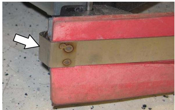
8. Fasten the retaining band latch onto the side squeegee assembly.
