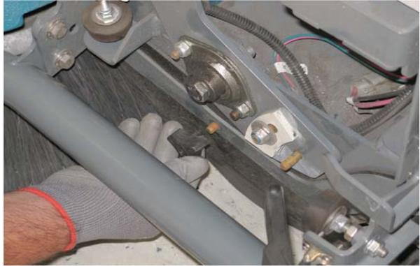
6. Remove the side skirt plate and side skirt from the Pre-Sweep assembly.
