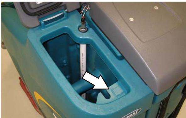
3. Fill the recovery tank with water (not to exceed 60°C / 140°F). Fill the recovery tank to just above the top of the ES filter.
