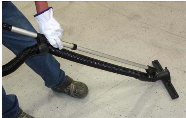
7. When finished vacuuming, press the *Vacuum fan/squeegee button* to turn off the vacuum fan. The squeegee will raise.
