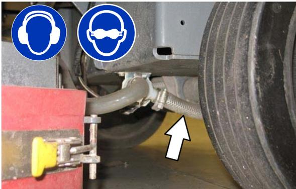
4. Use between 13.8 – 27.6 kPa (2 – 4 psi) of compressed air to blow remaining solution from the disconnected hose.
