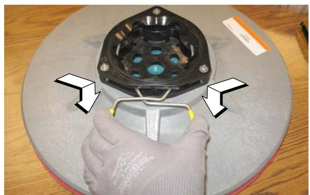
7. Place the new side brush underneath the side brush assembly and lift the side brush up onto the side brush hub until the brush locks onto the hub.
