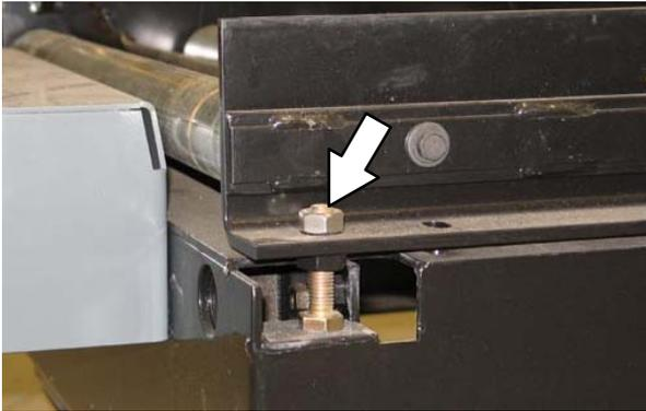
Raise battery cart rollers: Use a wrench to loosen the jam nut and turn the bolt clockwise. Retighten the jam nut.
