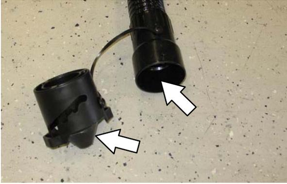
7. Twist the drain cuff closed and hook the drain hose back onto the solution tank.
