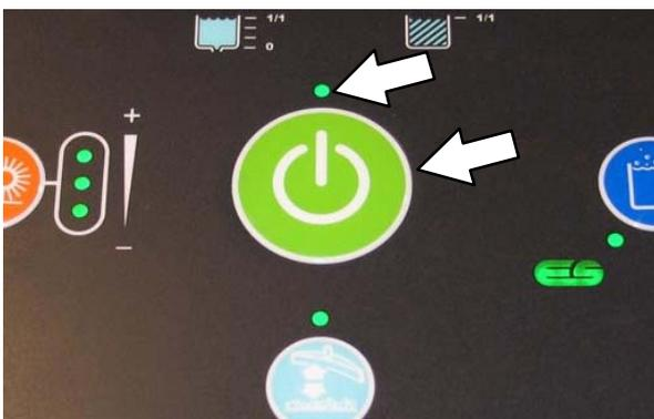
6. Repeatedly press the *Solution increase* button (+) until the solution flow is at the highest setting.
