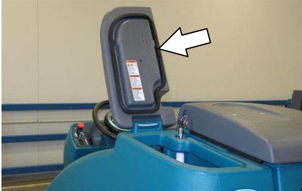
2. Fill solution tank with water (not to exceed 60°C / 140°F). Fill the solution tank with water until the level is approximately 50 mm (2 in) below the indicator tab.
