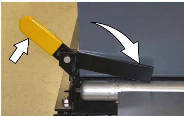
10. Raise the rollout battery retainer plate to release the battery cart from the machine.
