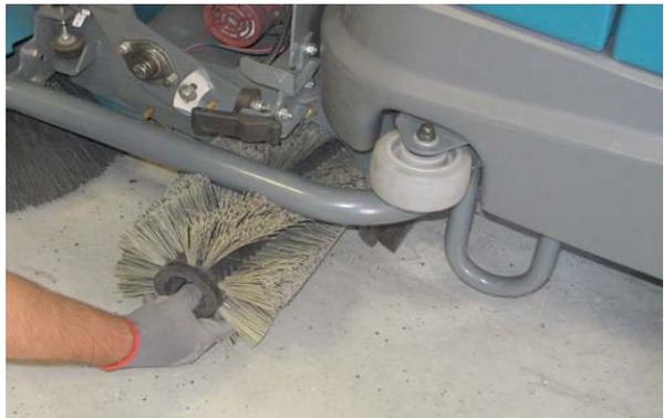
8. Guide the slotted end of the new brush onto the drive hub.
