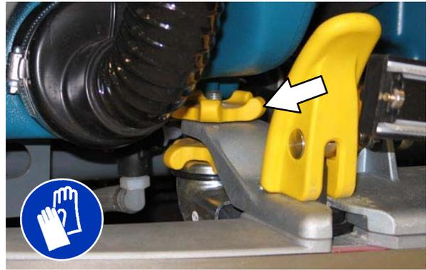
4. Turn the adjustment knobs counterclockwise to increase deflection or clockwise to decrease deflection.
