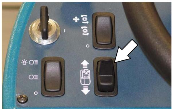
**NOTE:** An audible alarm will sound when the *Directional switch* is placed into reverse.
