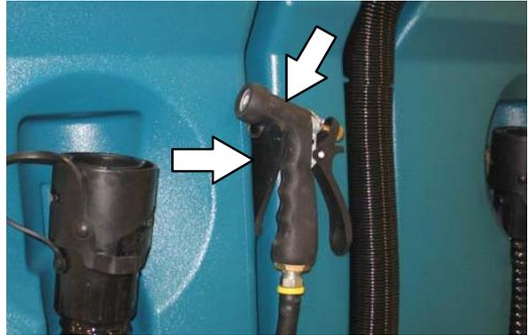
6. Press the bottom of the *Spray nozzle switch* to turn off the water supply. The light on the switch will turn off when the spray nozzle is turned off.
