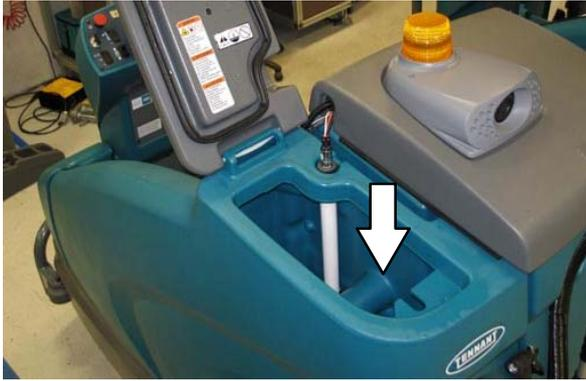
11. Place the *ec-H2O* system outlet hose into an empty container.
