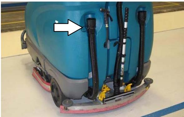
3. Hold the drain hose near a floor drain, twist the drain nozzle open, and place the hose near the floor drain.
