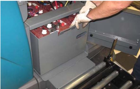
9. Pull up on the handle to lower the cart battery stop bar. This will keep the batteries from rolling off the cart.
