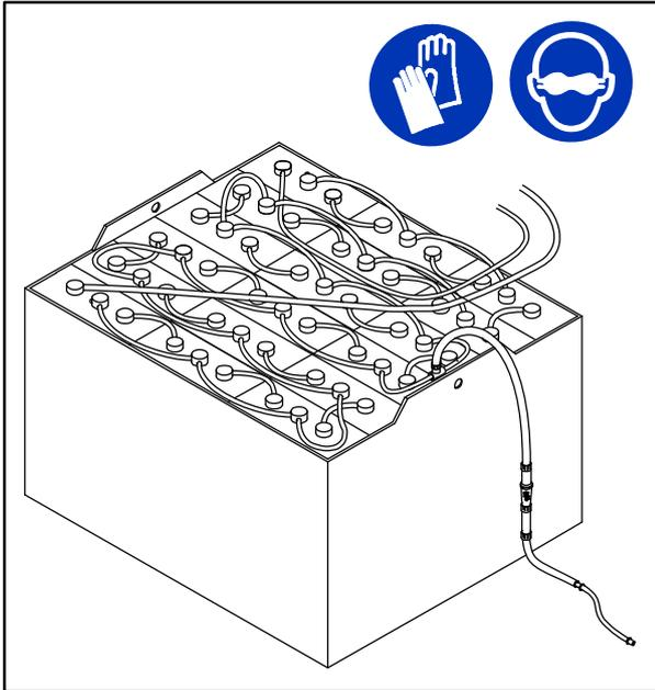
Check for the battery watering system hoses and connections for damage or wear after every 100 hours.
