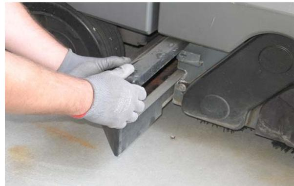
**NOTE:** The scrub head must be lowered approximately 25 mm (1 in) to remove debris trough.
