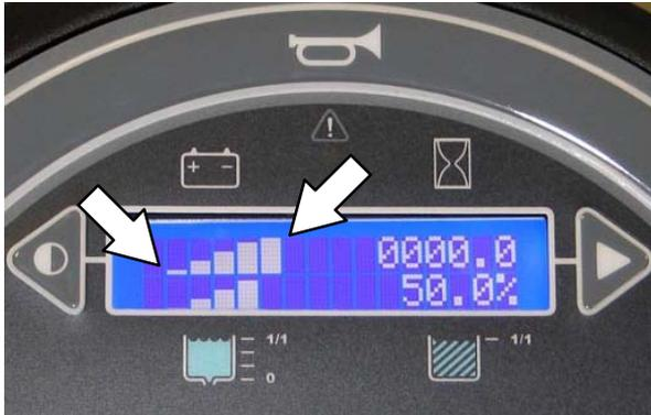
When the batteries are fully charged, all five bars are lit. Recharge the batteries when there are no longer any bars shown in the display.
