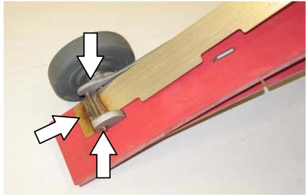
15. Install the retainer along the rest of the squeegee assembly and fasten the latch onto the other end of the squeegee assembly.
