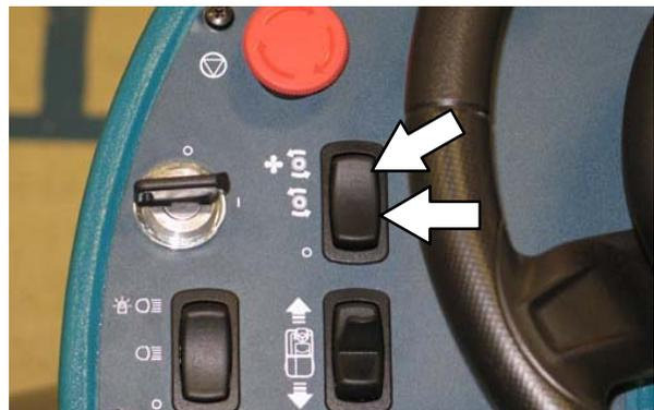
4. Press the bottom of *Pre-Sweep switch* to shut off the Pre-sweep system and dust control system.
