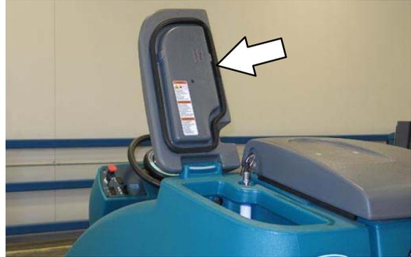
2. Fill the solution tank with only clean COOL WATER (less than 21°C / 70°F). DO NOT use hot water or add any conventional floor cleaning detergents or a FaST or ec-H<sub>2</sub>O system failure may result. Fill the solution tank with water until the level is approximately 50 mm (2 in) below the indicator tab.
