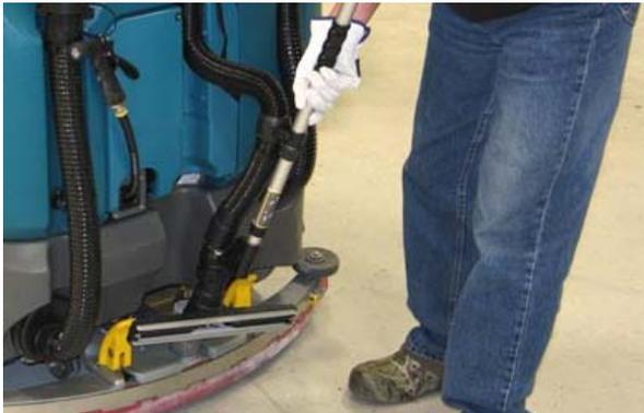
3. Insert the vacuum wand cap into the vacuum port in the vacuum wand.
