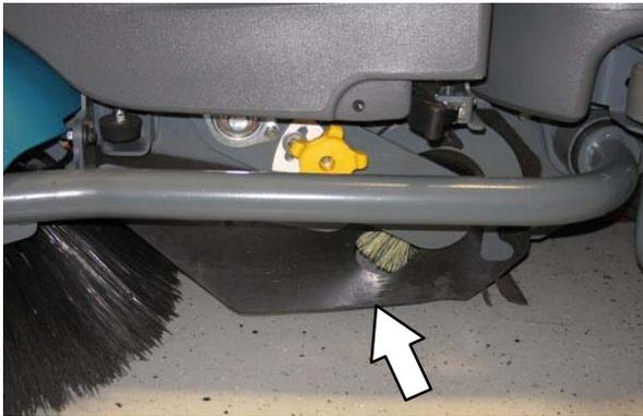
Check the skirts for damage and wear after every 50 hours of operation.
