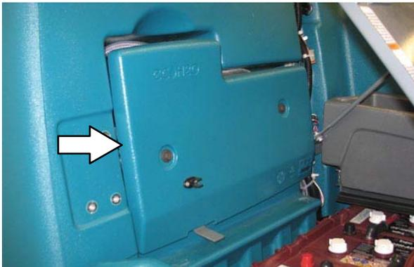
3. Remove the drain hose from the ec-H<sub>2</sub>O compartment.
