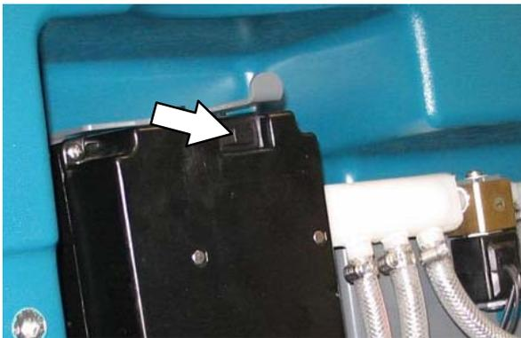
13. Disconnect the drain hose from the *ec-H2O* manifold hose.
