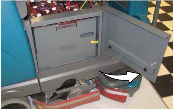
3. Disconnect the machine connector from the batteries.
