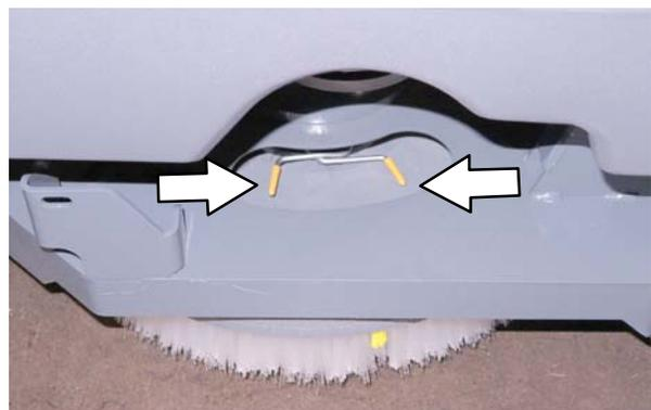
5. Squeeze the spring handles and let the brushes drop to the floor. Remove the brush from under the scrub head.
