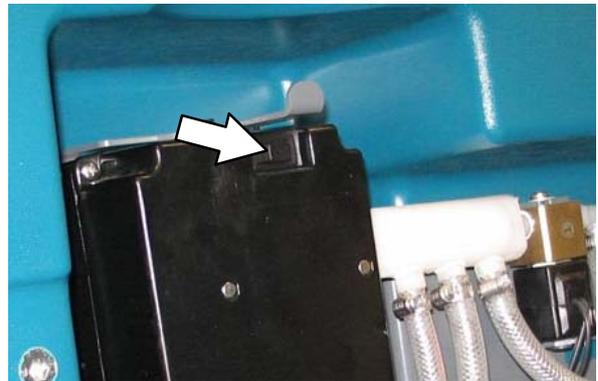
8. Press the *ec-H2O* module flush switch to shut off the system.
