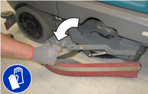
3. Unhook the retaining band latch from the side squeegee assembly.
