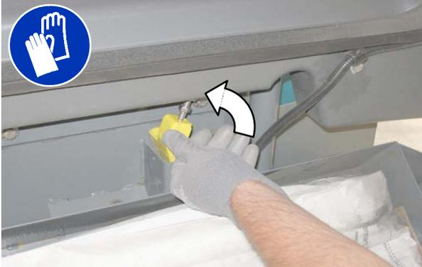
2. Remove the debris hopper from the Pre-Sweep assembly and empty the hopper.
