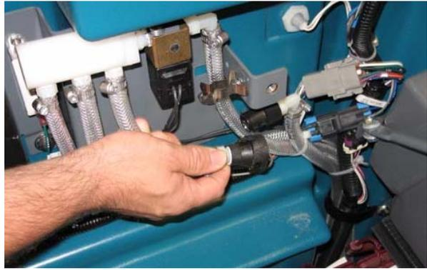
5. Place the drain hose into an empty container.
