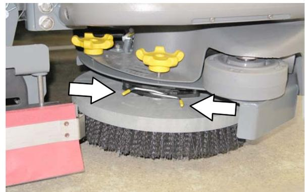
5. Remove the side brush from under the side brush assembly.
