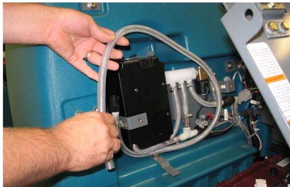
4. Disconnect the outlet hose from the hose connected to the ec-H<sub>2</sub>O manifold.
