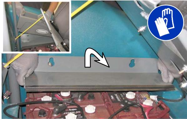
4. With adequate assistance carefully install the batteries into the battery compartment tray and arrange the battery posts as shown. Insert the foam spacers along side the batteries as shown if installing the smaller batteries.
