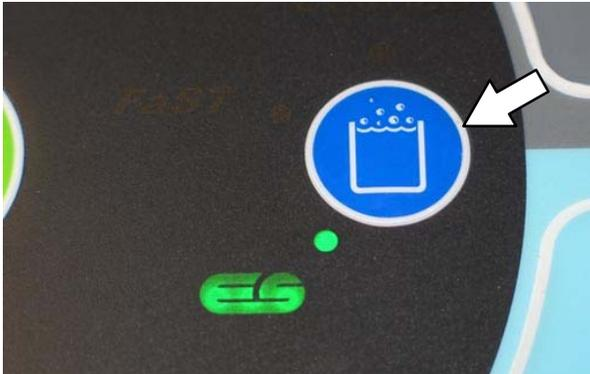
*NOTE: When the ES system is turned on there is a slight delay before the ES pump begins operating.*
