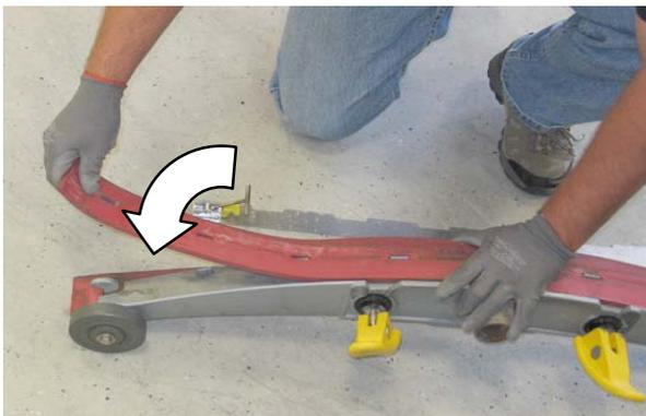
14. Insert the hinge end of the retainer into the hooks in the inner frame.
