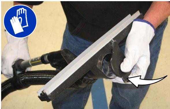
4. Twist the vacuum nozzle to the vacuum position and extend the handle to the desired length.
