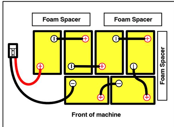
5. Using the supplied battery post boots, connect the cables to the battery posts, RED TO POSITIVE (+) & BLACK TO NEGATIVE (-).
