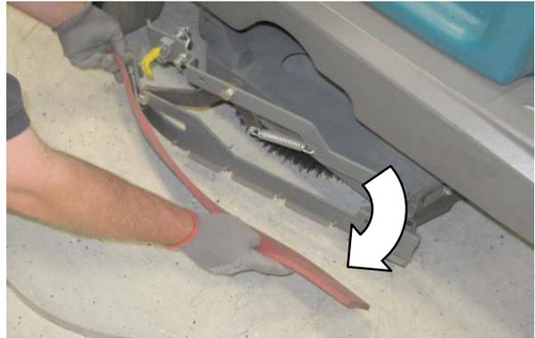
6. Install the rotated or new rear squeegee blade onto the side squeegee assembly.
