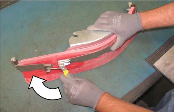
8. Reinstall the side brush squeegee assembly onto the side brush assembly.
