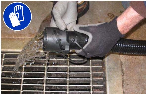
4. If necessary, twist the drain nozzle to another position to adjust the flow rate.
