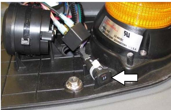
If the overload that caused the circuit breaker to trip is still present, the circuit breaker will continue to stop current flow until the problem is corrected.
