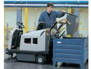
Hand-assisted high dump up to a maximum height of just over 3 ft.
