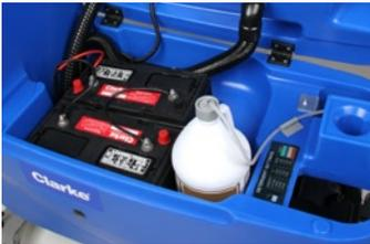
Easy access to battery compartment is great for maintenance and installation. Choose either 130 AH wet or 114 AH AGM batteries.
