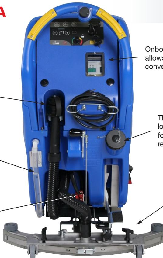
Onboard battery charger allows charging at any convenient electrical outlet
