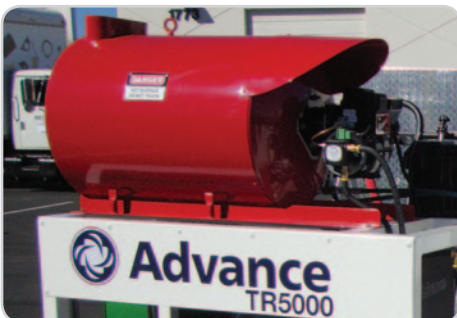
An optional, diesel-fueled water heater provides heated water for even more aggressive cleaning.
