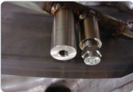
The location of the spray tips—pointed straight down near the surface—ensures pressurized water contacts the surface with maximum cleaning power.
