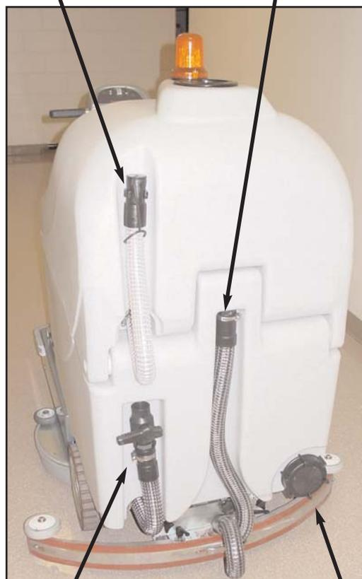
**Recovery Tank Discharge Hose and Valve**
