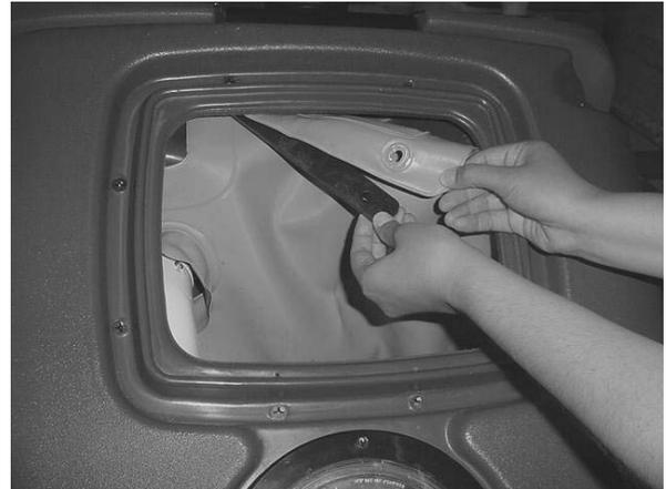
3. Angle mandrel and bag into tank fitting toward front of machine. Push mandrel into fitting until it bottoms out.
