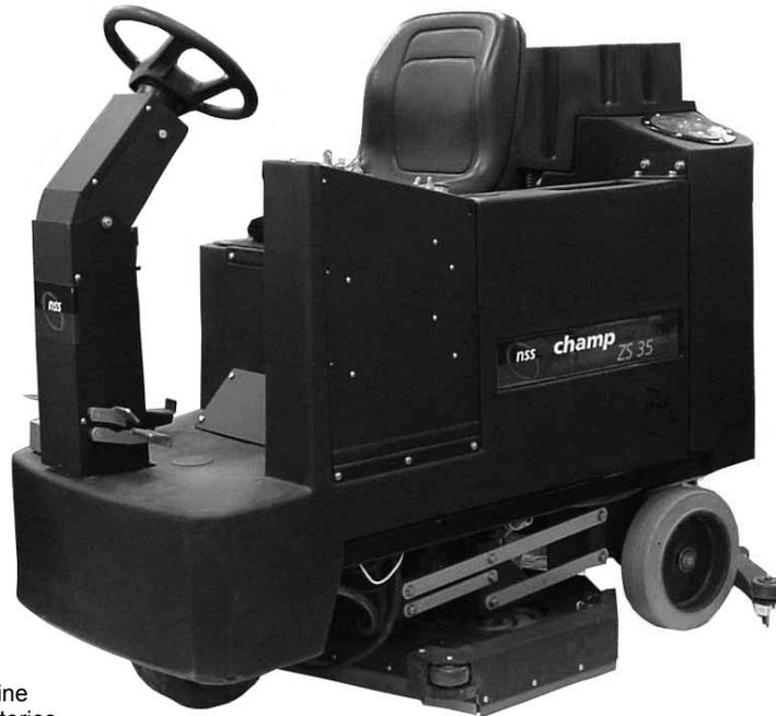
The 46-in. curved squeegee funnels dirt and water into the center of the assembly, where it is picked up by the powerful vacuum motor. Waterlift on the Champ 3529 is rated at 80 inches.
