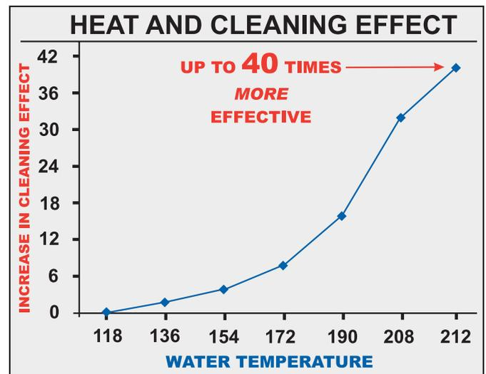
Increasing solution temperature up to 212° F at the spray tip dramatically improves cleaning results.
