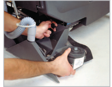
Brush deck slides out 5 in (13 cm) for edge cleaning
