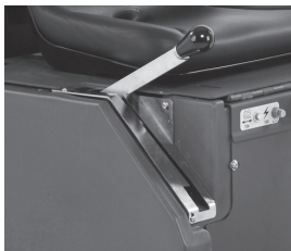
Mechanical deck lift lever.
