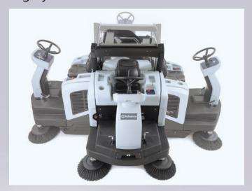
Front steering and front wheel drive with tight turning radius.
