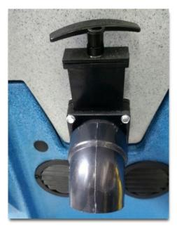
**NOTE:** Remove the elbow if you will be loading the machine into a vehicle to prevent damage to the elbow and to the drain valve.
