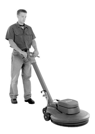
At 2000 rpm, the Whirlamatic™ 20 Ultra can give your floors a mirror-like shine in one pass. And unlike other burnishers that adjust pad pressure with a front-mounted caster, the Whirlamatic™ 20 Ultra uses a gas shock. This gas shock, a flexible pad holder and an exclusive pivoting motor keep the pressure evenly distributed against the contours of your floor so 100% of the pad makes contact at all times, whether the surface is even or uneven. The result is a consistent luster in less time.
