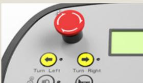
Press the turn signal buttons to activate the left and right turn signals.
