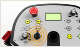
Insert the operator key, and turn to start the sweeper.
