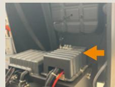
3. Open the machine cover and check the broom circuit breakers.
