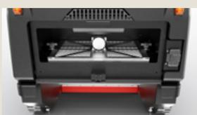
Remove the rear filter panel to check the filter, reinstall panel and hopper.
