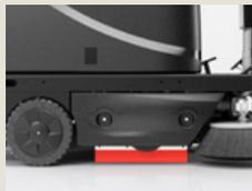
1. Check if all blades are correctly adjusted and not damaged.
