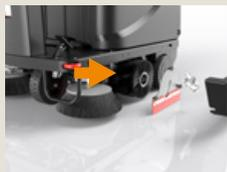
1. Make sure main broom is turning and not worn out. Adjust broom height if needed.
