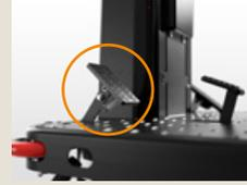
4. Check if the parking brake pedal is engaged.
