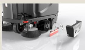
Remove, clean and inspect the main broom and check the side brooms. Clean the machine with a wet cloth.
