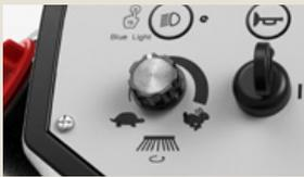
Adjust the speed of the side brooms by changing the side broom speed knob.
