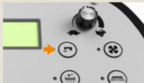
Press the water misting button to activate the side broom dust control.
