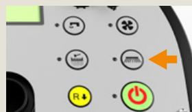
Press the side broom button to lift the side brooms and use the machine with only main broom.
