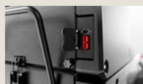
Charge the machine using the rear charging connection. It has two connections, one for external charger and one if on-board charger is installed.
