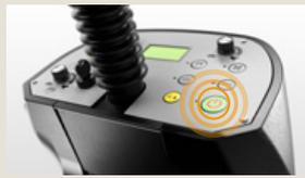
Press the OneTouch™ button to enable all sweeping functions, the brooms will lower automatically.
