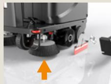
2. Adjust the side broom if needed, replace the side broom if bristles are worn out.
