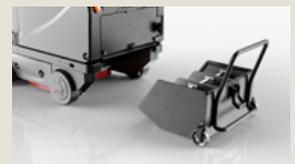
Press the OneTouch™ button to stop all functions. Slowly release the hopper locking mechanism as it may be heavy. Use the handle to remove and empty the hopper.
