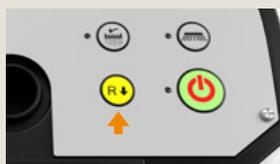
Press the reverse button to move the sweeper backwards. Machine does not sweep in reverse.
