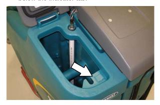
3. Fill the recovery tank with water (not to exceed 60°C / 140°F). Fill the recovery tank to just above the top of the ES filter.
