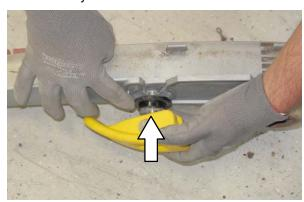
13. Place the rotated or new squeegee blade onto the inner frame. Be sure the squeegee is securely attached on each tab on the inner frame.
