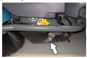
Check the skirts for damage and wear after every 50 hours of operation.
