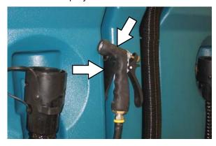
6. Press the bottom of the *Spray nozzle switch* to turn off the water supply. The light on the switch will turn off when the spray nozzle is turned off.
