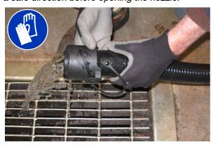
4. If necessary, twist the drain nozzle to another position to adjust the flow rate.
