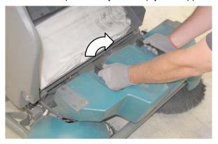
Reinstall the debris hopper into the Pre-Sweep assembly.
