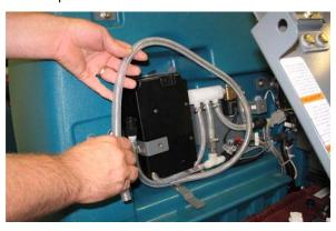
8. Disconnect the outlet hose to the scrub head from the ec-H2O manifold hose.
