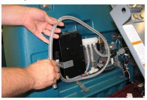
4. Disconnect the outlet hose to the scrub head from the ec-H2O manifold hose.
