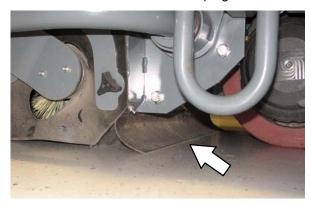
Check the skirt for damage and wear after every 50 hours of operation.
