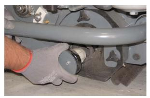
5. Remove the three knobs holding the Pre–Sweep side skirt and side skirt plate to the Pre–Sweep assembly.
