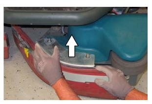
4. Loosen the retaining band latch.
