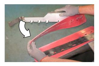
NOTE: The squeegee blade(s) have two sets of slots for adjusting the squeegee blade deflection. Install / reinstall squeegees so the deflection is approximately 12 mm (0.50 in) for smooth floors and 15 mm (0.62 in) for rough floors.
