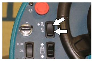
4. Press the bottom of *Pre–Sweep switch* to shut off the Pre–sweep system and dust control system.
