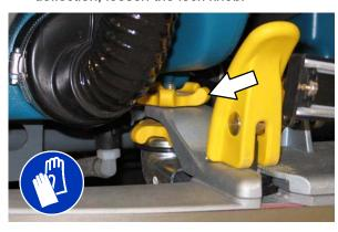
4. Turn the adjustment knobs counterclockwise to increase deflection or clockwise to decrease deflection.
