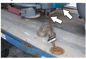
The rear tie-down locations are the holes in the frame.
