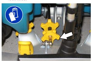
5. Turn the squeegee tilt adjust knob counter-clockwise to decrease the deflection at the ends of the squeegee blade.
