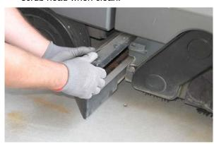
NOTE: The scrub head must be lowered approximately 25 mm (1 in) to remove debris trough.
