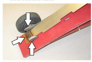
15. Install the retainer along the rest of the squeegee assembly and fasten the latch onto the other end of the squeegee assembly.
