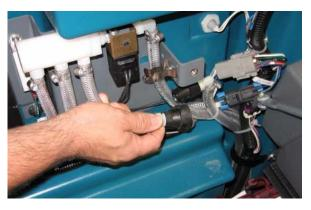
9. Connect the drain hose to the ec-H2O manifold hose disconnected from the outlet hose in the previous step.
