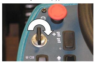
9. Press and release the ec-H2O module flush switch to start the flush cycle.
