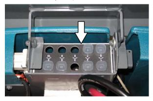
Circuit breakers 11 through 19 are located on the electrical panel.
