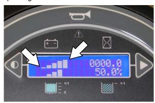
When the batteries are fully charged, all five bars are lit. Recharge the batteries when there are no longer any bars shown in the display.
