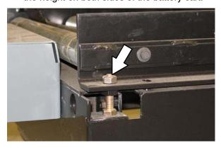
Raise battery cart rollers: Use a wrench to loosen the jam nut and turn the bolt clockwise. Retighten the jam nut.
