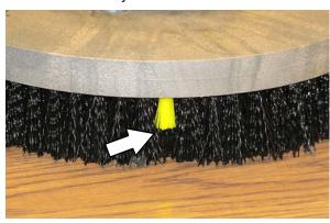
Cleaning pads must be placed on pad drivers before they are ready to use. The cleaning pad is held in place with a center disk. Both sides of the pad can be used for scrubbing. Turn the pad over to use the other side.
