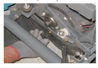
6. Remove the side skirt plate and side skirt from the Pre-Sweep assembly.
