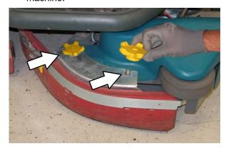
4. Squeeze the spring handles and let the side brush drop to the floor.
