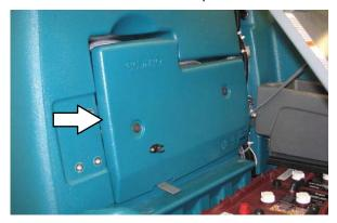
Remove the drain hose from the ec-H2O compartment.
