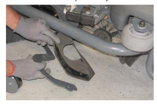
7. Remove the cylindrical brush and replace with a new brush.
