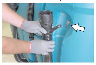
Check the vacuum fan inlet filter daily. Clean inlet filter with a damp cloth or hose when dirty. Allow filter to completely dry before reinstalling it into the machine.
