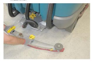
5. Loosen the retainer latch and remove the retainer from the squeegee assembly.
