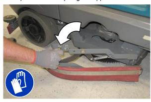
3. Unhook the retaining band latch from the side squeegee assembly.
