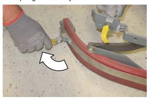
4. Remove the retaining band from the side squeegee assembly.
