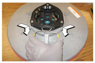
Push the new brush under the scrub head, align the brush drive socket with the brush drive hub, and lift the brush up onto the brush drive hub until the brush locks onto the hub.
