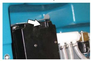
NOTE: The module will automatically shut off when the flush cycle is complete (approximately 7 minutes). The module must run the full 7 minute cycle in order to reset the system indicator light and alarm.
