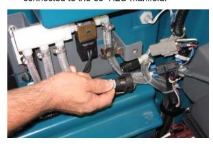
5. Connect the drain hose to the ec-H2O manifold hose disconnected from the outlet hose in the previous step.
