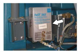
Remove the perforated knock outs from the new FaST-PAK carton. DO NOT remove the bag from the carton. Pull the hose connector from the bottom of the bag and remove the hose cap from the connector.
