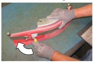
8. Reinstall the side brush squeegee assembly onto the side brush assembly.
