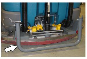
To engage the rear squeegee protector, pull the pin, lower the protector bar, and reinsert the pin.
