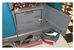
3. Disconnect the machine connector from the batteries.
