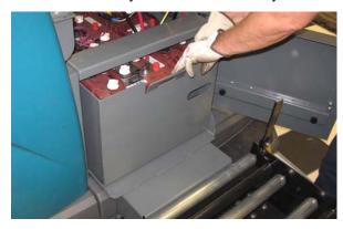
9. Pull up on the handle to lower the cart battery stop bar. This will keep the batteries from rolling off the cart.
