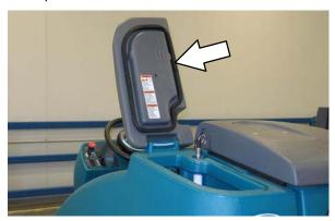
2. Partially fill solution tank with water (not to exceed 60°C / 140°F). Pour the required amount of detergent into the solution tank. Continue filling the solution tank with water until the level is approximately 50 mm (2 in) below the indicator tab.
