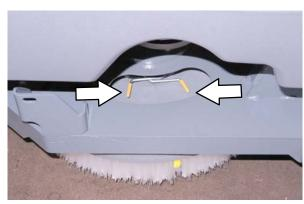
5. Squeeze the spring handles and let the brushes drop to the floor. Remove the brush from under the scrub head.
