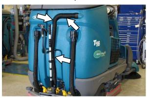
12. Snap the vacuum wand lanyard onto the solution tank to secure the vacuum wand / squeegee vacuum hose to the machine.
