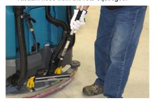
3. Insert the vacuum wand cap into the vacuum port in the vacuum wand.
