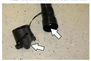
7. Twist the drain cuff closed and hook the drain hose back onto the solution tank.
