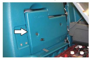
3. Remove the drain hose from the ec-H2O compartment.
