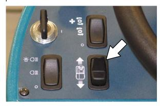
NOTE: An audible alarm will sound when the Directional switch is placed into reverse.
