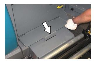
6. Step on the left side of floor lock to set the battery cart floor lock.
