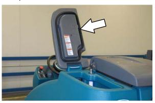
Fill the solution tank with only clean <u>COOL</u> <u>WATER</u> (less than 21°C / 70°F). DO NOT use hot water or add any conventional floor cleaning detergents or a FaST or ec-H2O system failure may result. Fill the solution tank with water until the level is approximately 50 mm (2 in) below the indicator tab.
