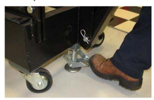
7. If necessary, adjust the height of the battery cart rollers. The battery cart rollers must be level with the machine battery rollers. Adjust the height on both sides of the battery cart.
