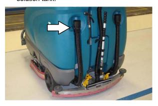
3. Hold the drain hose near a floor drain, twist the drain nozzle open, and place the hose near the floor drain.
