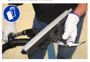
4. Twist the vacuum nozzle to the vacuum position and extend the handle to the desired length.
