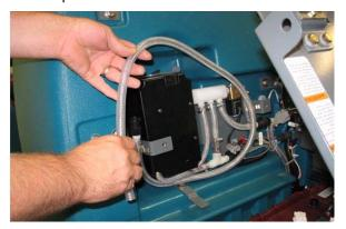
4. Disconnect the outlet hose from the hose connected to the ec-H2O manifold.
