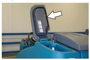
2. Fill solution tank with water (not to exceed 60°C / 140°F). Fill the solution tank with water until the level is approximately 50 mm (2 in) below the indicator tab.
