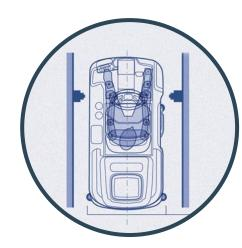
Both the SG28 and SG36 models were designed with the ability to easily drive through a standard 36-inch (91 cm) doorway to simplify transportation to and around the job site.
