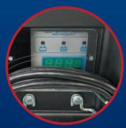
Onboard battery charger and charger cord is located on the rear of the machine. Access window provides battery and charger status.
