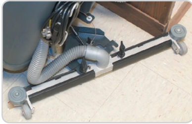
"Break-away" rear squeegee prevents damage to machine and facility.
