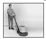
Built-in solution tank is made to hold 3 gallons (11.4 L) of cleaning chemical. Solution control lever allows chemical to flow through shower feed of brush or pad holder.
