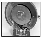
The high speed Matador machines feature Power-Flex™ transmissions which use a poly-V belt with grooved pulley. It's been field proven for years to be durable and virtually maintenance free.
