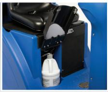
**Chemical mixing system** Optional, onboard chemical mixing system saves you money and time along with helping to save the environment. Every drop will be used to clean your floors and will be mixed at the correct proportion.
