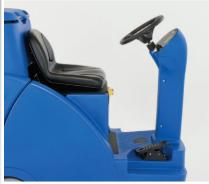
**Operator compartment** Open operator compartment with low-step height and angled floorboard allows easy on/off boarding.
