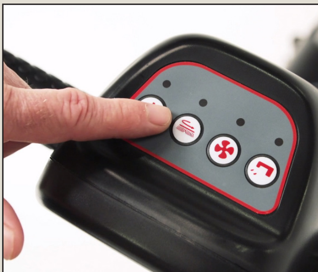
Switch on start, brush, vacuum and water
