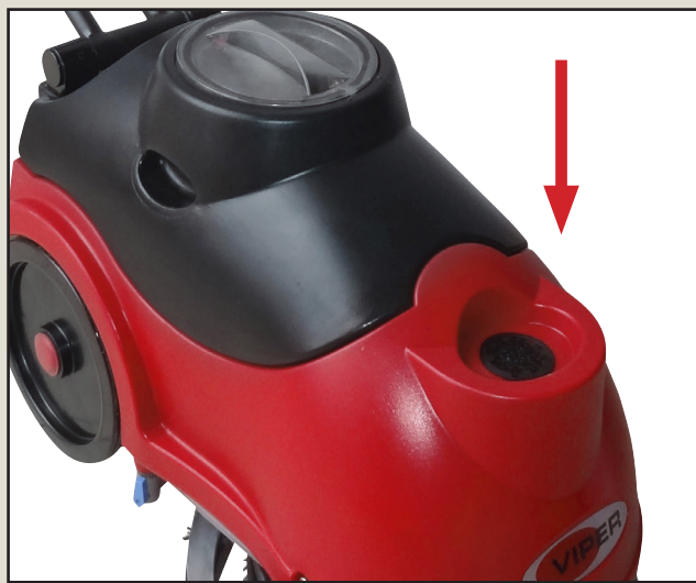
Fill water tank with fresh water. Add low foam detergent
