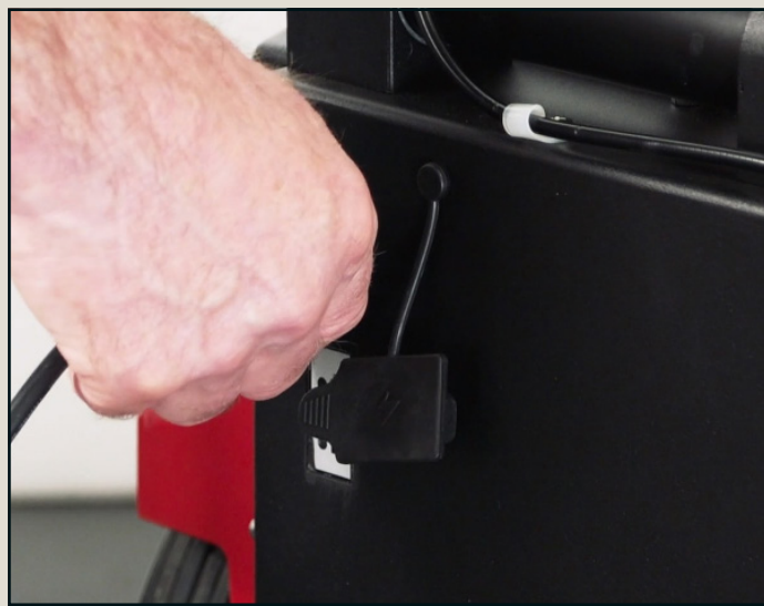
Connect battery charger to socket
