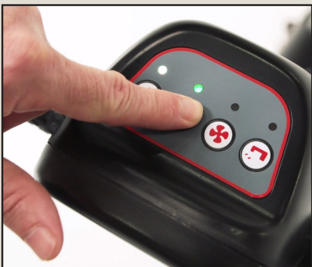
Switch on start, brush, vacuum and water
