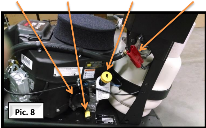
Oil Filter-Oil Drain Plug-Oil Dipstick/Fill-Battery connector Starting Solenoid-Starter-Bonnet filter-air Filter Cover
