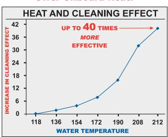
Increasing solution temperature up to 212° F at the spray tip dramatically improves cleaning results.
