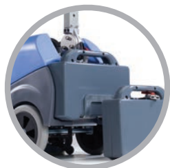
Environmentally preferred gel battery easily removed for transport
