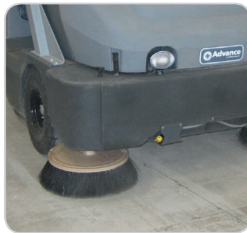
DustGuard™ suppresses side broom generated dust allowing continuous use, and increasing, dust controlled productivity by over 70%.
