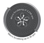
Patented REV™ random orbital scrubbing technology with high speed 1/4 inch micro scrubbing and 14 inch rotational macro scrubbing attacks dirt from multiple directions for superior cleaning effectiveness.
