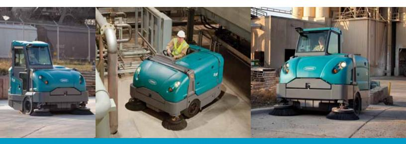
Engineered for reliable, industrial-strength sweeping, the Tennant S30 rider sweeper improves indoor and outdoor performance, significantly reduces sound levels and features the exclusive SweepSmart™ dust control system.
