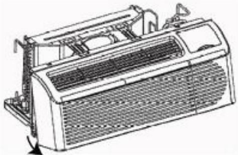
3. Place a Shower cap over the switch panel to protect electronics.
