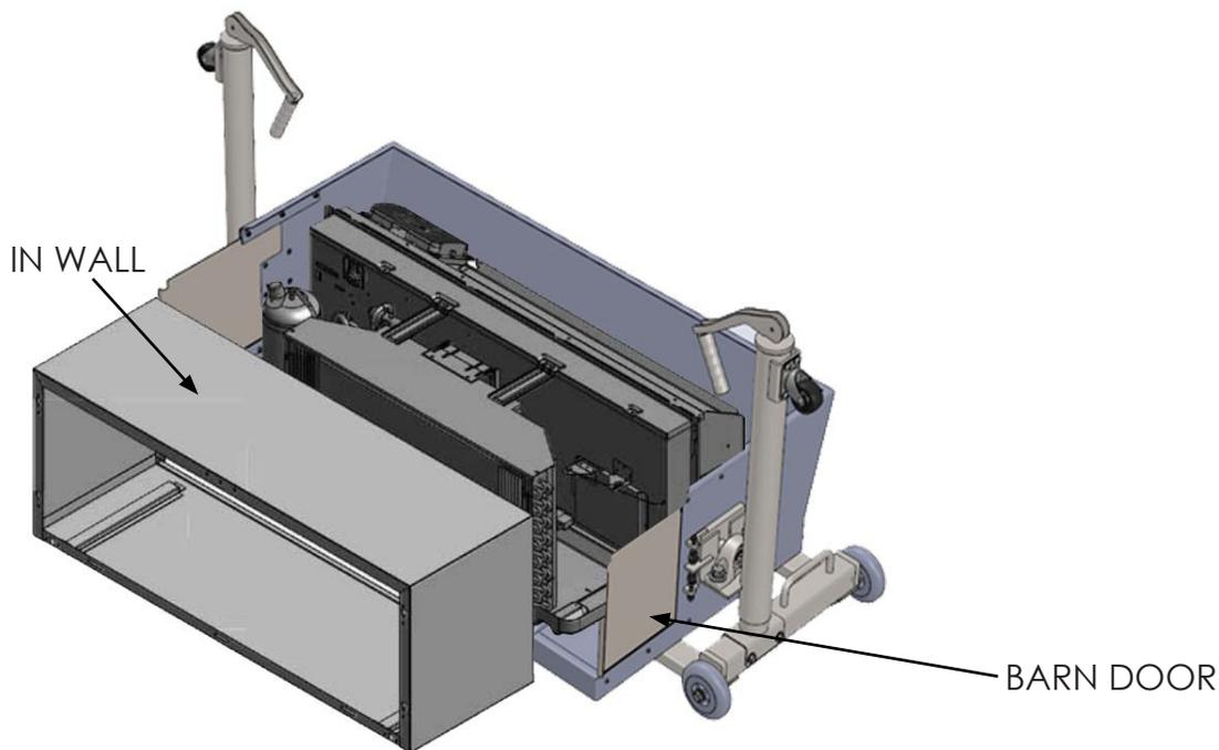
11. Using your 2 gallon chemical sprayer with pre mixed chemical, spray the rear condenser, pan, front evaporator core, heating element, side filter and any part of the fan that is accessible. Do not spray the switch panel.
