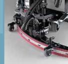
Its shape is of significant importance as its primary function is to pick up dirty water with the aid of a vacuum motor. It is, in fact ,when the drying takes place that that work is optimised, as when one eliminates the soiled water all that is guaranteed to remain is a brilliantly clean and shiny surface. Other important variables that were taken into consideration when designing the squeegee were: materials chosen, parabolic shape, variable positioning points.
