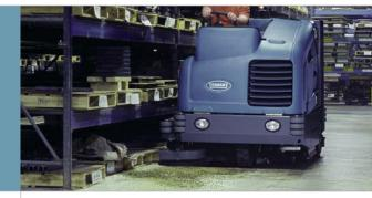
The first fully-integrated scrubber-sweeper, the M20 is engineered for consistent, industrial-strength cleaning whether scrubbing, sweeping or doing both at once.
