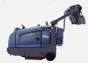
Cleaning productivity is increased with a large 3.9 ft $^3$  / 110 liter, 390 lb / 177 kg debris hopper with 60 in / 1,520 mm variable dump height.
