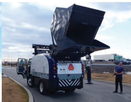
LEFT Joystick controlled robotic vacuum hose arm collects debris in hard to reach areas and safely vacuums up trash cans.
