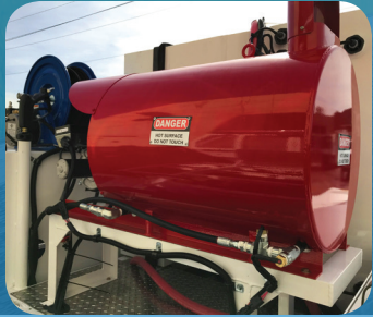
Diesel-fueled water heater for an aggressive deep clean.
