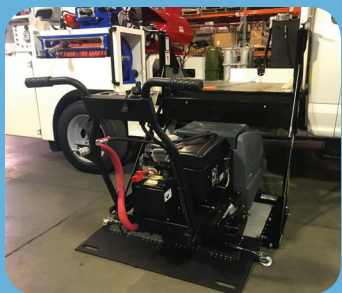
Automatic lift gate for quick and easy loading and unloading of CY210 walk behind cleaning system.
