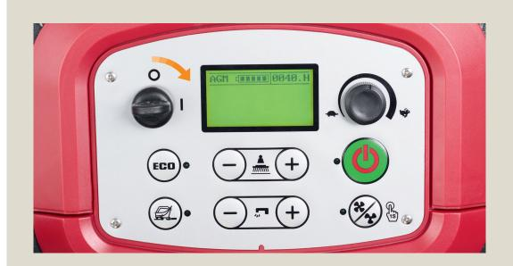
Turn on the key and verify there is enough battery power to complete the work. Charge batteries if required.
