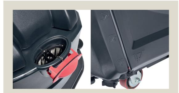
Remove the red cover and fill the tank with water, max temperature 40C/104F. Add appropriate low foaming detergent. Maximum tank capacity 85L/22Gal. Check solution level with red ball on the side of the machine.
