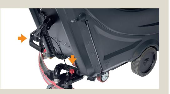
**Disc version:** install the brushes/pad holders manually, then press the One button start icon to enable scrubbing. The deck will lower automatically, and the vacuum will start.
