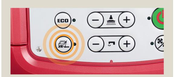
Press the Floor Finish Removal icon (orbital only) for removing finish: pad pressure will be set to maximum, solution flow will be set to minimum & machine speed will be held at 1.0 km/h (0.6 mph).
