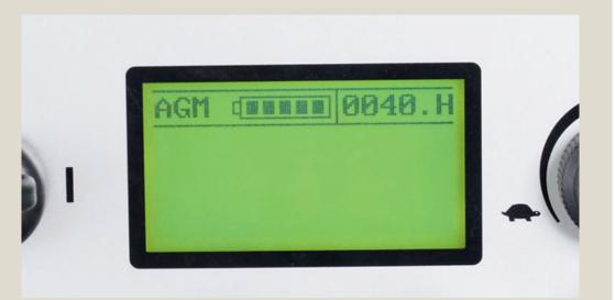
**Daily:** Charge the machine at the end of the cleaning shift or if the battery indicator is low or showing empty.
