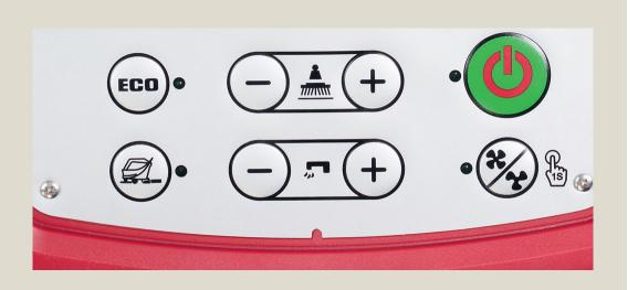
Press the + or – buttons to increase / decrease the water flow rate and/or brush pressure.
