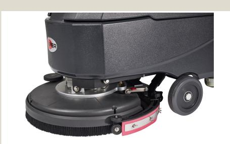
Place the brush or the pad-holder under the deck and Lower the deck or the brush/ pad holder by pressing the pedal. The squeegee is raised and lowered with the deck.
