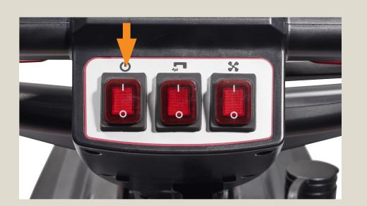
Connect the power supply plug to the electrical mains and press machine ON button.
