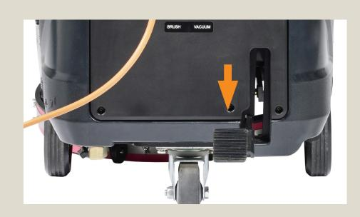
Lift the deck by pressing the pedal.
