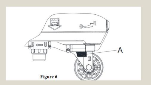
Solution flow can be adjusted according to the scrubbing need
