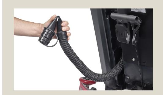
**Daily:** Empty the recovery tank using the recovery empty hose. Bend the soft part before removing the cap to control the flow.
