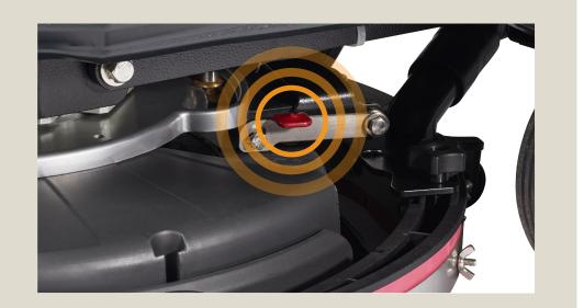
Lift the squeegee up by hand until it locks in up position and turn suction off for double scrubbing.
