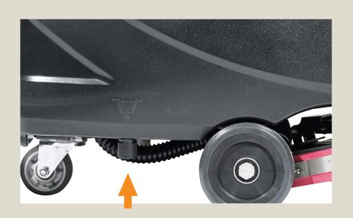
**Daily:** Empty the clean water tank using the solution tank drain knob under the machine.
