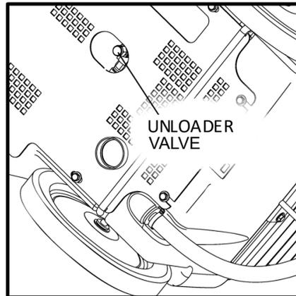
11. From the factory your machine is set to spray at 600 psi (high pressure) and 200 psi (low pressure w/chemical injection). To lower pressure turn the unloader valve knob counter clockwise. The valve is accessed from below the machine through a hole in the bottom frame. Only turn the valve a maximum of three revolutions.
