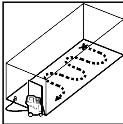
4. Position the machine in the doorway, lock front casters. Start at furthest point in the room and work towards the door.
