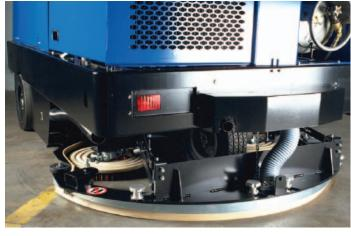
Patented Accu-Track™ squeegee provides superior water pick-up even during the tightest turns.
