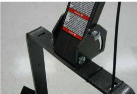
8. Place the washer and handle adjustment lever on the bolt. Thread the adjustment lever in until it is against the handle bracket, but do not tighten.
