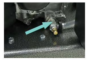
**Note:** In order for the oil to drain, it may be necessary to loosen the oil fill cap.
