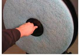
**CAUTION!** Carefully inspect the pad holder for cracks or damage. Replace if necessary.
