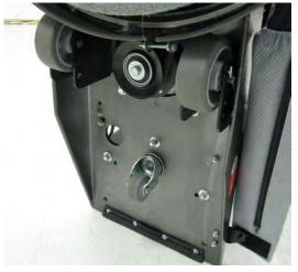
**NOTE:** To increase pad pressure (more aggressive) move wheels to rear of machine. To decrease pad pressure (less aggressive) move wheels toward the front of machine.
