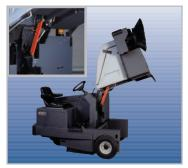
The 15 ft³ (425 L) hopper holds up to 1,200 lb (544 kg) and hydraulically lifts up to 60 in (152 cm) to dump.
