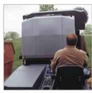
Hopper safety features include support strut (red), cover safety latch, hopper-up speed control, and visibility with hopper up.
