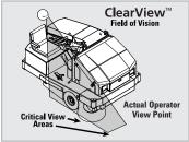
The unique off-set hopper gives the operator a view of critical areas, essential when sweeping along walls or curbs and when maneuvering in close spaces.
