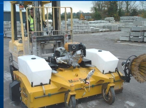
Model 425 including gasoline engine, gravity water system and side brush
