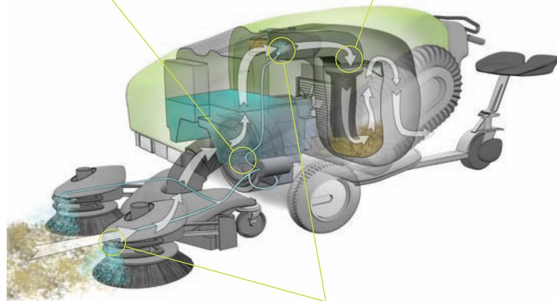
**3** Water Dust Control System. Spray jets located on each of the 400 Series sweeping brushes and inside the suction tube provide added dust control and can be used to dispense a fragrance in the work area.
