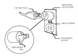
A grounding adapter must be installed as shown here if only two-prong outlets are available. The outlet box must be grounded and the grounding tab (or wire) on the adapter must be installed under the head of the screw in the center of the outlet cover. Grounding adapters for 120 volt plugs are available at most hardware stores.
