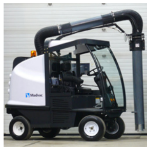
LEFT The ergo robotic joystick controlled vacuum arm results in productivity 6 times faster than a manual picker.
