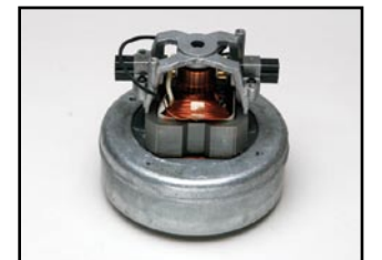
G12003 Backpack Vacuum Motor-High Air Flow 98" Waterlift, 120V, 5.7" FR, 5" overall height
