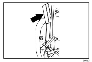
Raise Squeegee and Stop Vacuum: Pull the lever towards you, and move it to the right to lock the lever in the up position.
