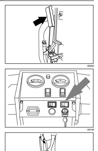
Squeeze the solution lever on the power wand to spray solution on the floor. Scrub 9. the floor with the brush side of the cleaning tool.
