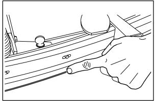
5. If the deflection is not the same over the full length of the blade, turn the squeegee leveling knob counter-clockwise to decrease the deflection at the ends of the squeegee.
