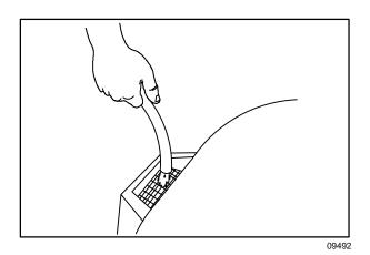
6. ES  $^{\text{\tiny M}}$  mode: Open the recovery tank cover.
