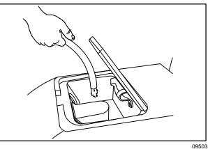
8. ES  $^{\text{\tiny M}}$  mode: Close the recovery tank cover.
