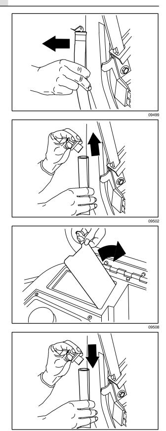
16. ES<sup>™</sup> mode: Place the solution tank drain hose back into the mounting clip.
