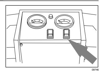
5. Start and lower the scrub brush with the scrub head release pedal.
