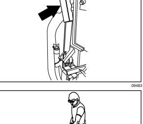
8. When finished, raise the squeegee to shut off the vacuum.
