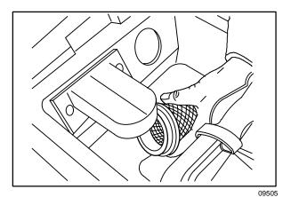
9. ES<sup>™</sup> mode: Rinse the ES<sup>™</sup> filter. Remove and clean the filter if it is still dirty. Put the filter back in the tank.
