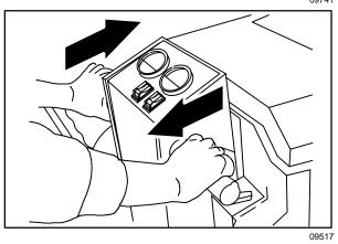
Stopping/Brush and Solution Off: Release the handles.
