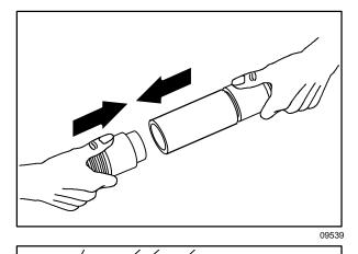
4. Attach the end of solution hose to the quick-disconnect. Push the connector in until it stops. Pull on the hose to make sure it is connected.
