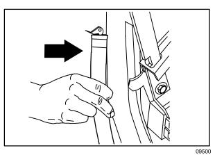
17. Close the solution tank cover, and lower the recovery tank. Rotate the stop arm out of the way to allow the recovery tank to close completely.
