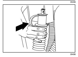
12. ES<sup>™</sup> mode: Remove the solution tank drain hose from the mounting clip.
