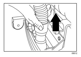
4. Connect the vacuum wand hose and the squeegee suction hose with the adapter.
