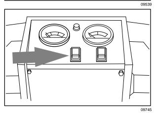
6. Lower the squeegee with the squeegee lever to turn the vacuum system on.
