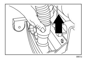
3. Connect the vacuum wand hose and the squeegee suction hose with the adapter.
