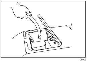
8. Rinse the float screen. Remove and clean the screen if it is still dirty. Put the screen back in the tank.
