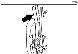
4. Start the solution flow with the solution switch.
