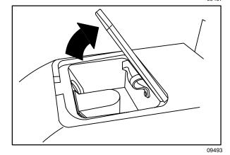
7. Flush out the inside of the recovery tank with clean water.
