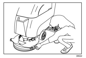
4. If the skirt needs to be adjusted, loosen the skirt band clamp and move the skirt up or down to touch the floor.
