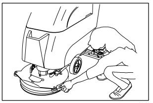
Check the squeegee for proper deflection. Check the squeegee blade for wear, rounded edges, nicks, or cuts.
