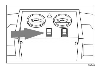
2. Release the machine parking brake, if your machine has this option.
