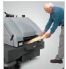
Hopper access door for hand-loading large items.
