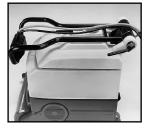
Handle bar adjusts to operator's comfort height, and folds over top of base for compact storage or easy carrying and transport.
