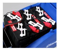
Battery compartment is easy to access. Battery options include either 195 Ah wet batteries or 234 Ah AGM batteries which feature long run times, longer life, and are totally maintenance free.
