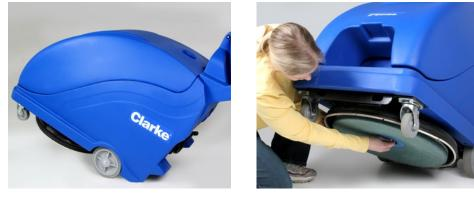
The operator can easily tilt back the machine for convenient pad change. The body features two molded foot areas for easy titling. There is also an angle-activated safety switch to prevent operation while in the tilted position.
